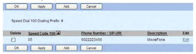
**STEP 7** To delete a Speed Dial 100 number, check the Delete box of the speed dial you wish to delete and click OK to save and return to the Outgoing Calls menu.
